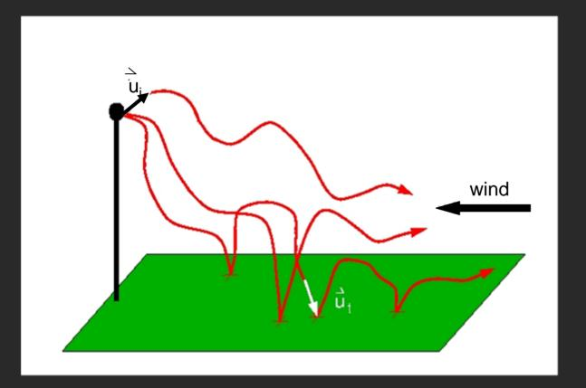
Start particle tracks at sensor location.
