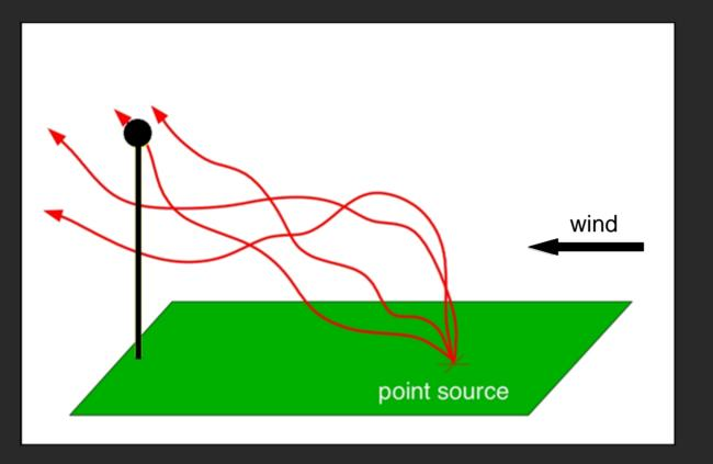
Evaluate many point sources and sample particle tracks at sensor height.
